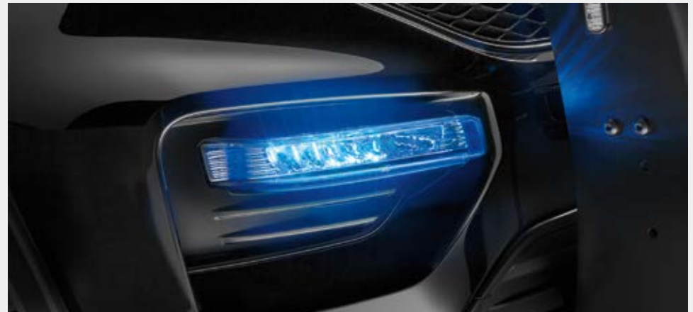
Front warning auxiliary lamps (21L).
